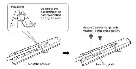
When securing the mounting plate, position the mounting plate depending on the desired height of the speaker.
